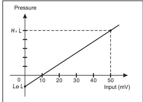
(1). When using the “Resistance Transmission Pressure Gauge” as the pressure sensor, the input signal parameter  $S_n$  must be set to  $PrE$ , set  $H_i L$  to the full scale value of the sensor, set  $L_{0L}$  to 0.
